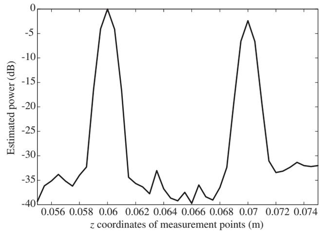
Fig. 14. Range resolution of the proposed imager at the center. Two point targets are placed for 0.06 and 0.07 m depths, and the resolution is acquired from a single transmit and receive event. The lines show the estimated power at the measurement points.
