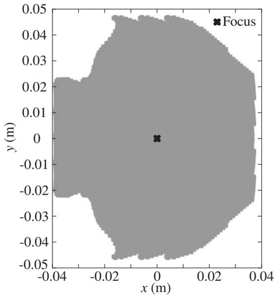
Fig. 13. Synthesized aperture from 14 transmit and receive events when measuring the center for a 0.07 m depth. The synthesized aperture is larger than a section of RGF; thus, the spatial resolution is improved utilizing the synthetic aperture technique.
