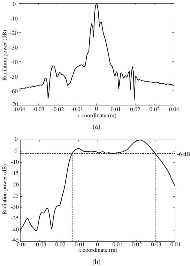
Fig. 10. Radiation pattern of the proposed imager in the  $x$ - $z$  section for (a) 0 m and (b) 0.07 m depths. The focus is set at the origin.
