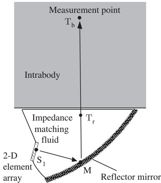
Fig. 8. Transmit pass in geometric optics. In geometric optics a transmit pulse from an element is reflected by the mirror, and then radiated to the measurement point  $T_b$  after passing through the focus  $T_r$ .
