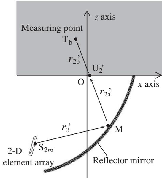
Fig. 4. Arrangement of a 2-D element array and a mirror in the numerical back-projection.
