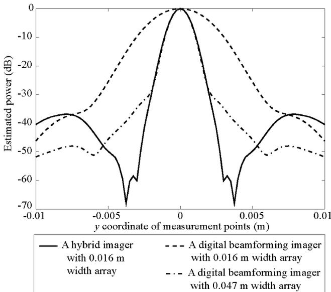
Fig. 16. Lateral resolution of the proposed imager with a 0.016 m width array and digital beamforming imagers with 0.016 and 0.047 m width arrays. A point target exists at the center for a 0.07 m depth, and lines show the estimated power at the measurement points in the  $y$ - $z$  section. The spatial resolutions of the proposed imager and digital beamforming imagers are improved, respectively, from 14 and 16 transmit and receive events.
