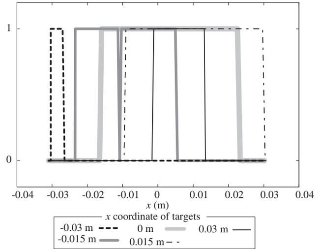
Fig. 11. Regions with a guaranteed focus on the  $x$  axis. The regions, whose  $x$  coordinates of measurement points are from  $-0.015$  to  $0.03$  m, contain the origin, and that whose  $x$  coordinate is  $-0.03$  m does not contain the origin. This corresponds to the radiation pattern shown in Fig. 10(b).
