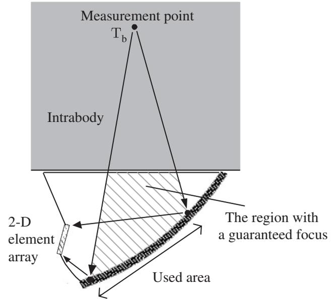
Fig. 9. Region with a guaranteed focus. When the focus is contained within the region, the transmit wave is radiated to the measurement point  $T_b$ .
