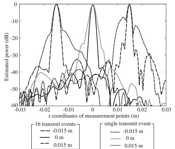
Fig. 15. Lateral resolution of the proposed imager acquired from single and 16 transmit and receive events in the  $x$ - $z$  section for a 0.07 m depth. A point target is placed at  $x = -0.015, 0, 0.015$  m in the  $x$ - $z$  plane for a 0.07 m depth. The lines show the estimated power at the measurement points.
