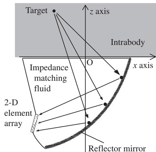
Fig. 1. Schematic view of the system in the receive phase.
