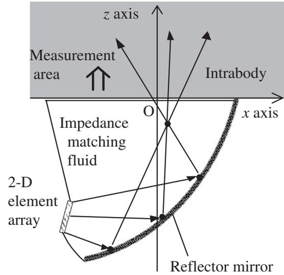
Fig. 2. Schematic view of the system in the transmit phase.
