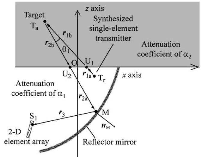
Fig. 3. Arrangement of a 2-D element array and a mirror in a transmit and receive event.
