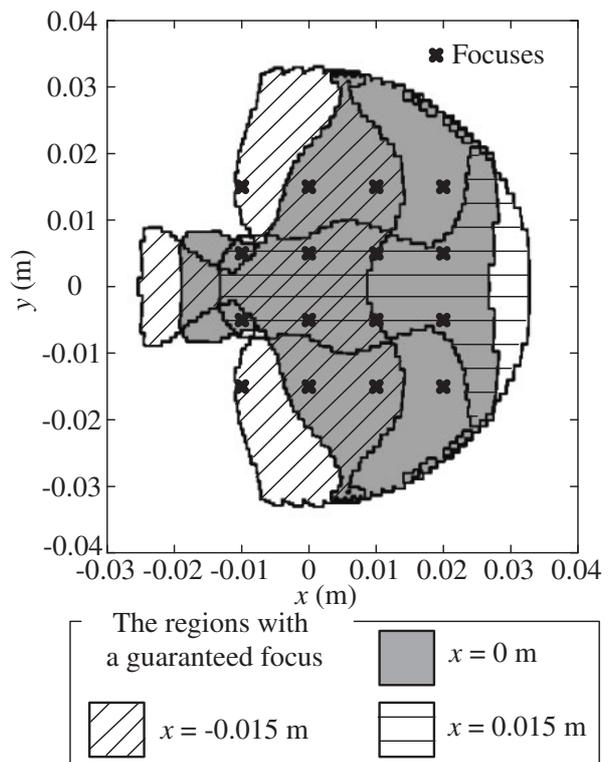
Fig. 12. Arrangement of the focuses and the regions with a guaranteed focus for a  $-0.01$  m depth. The RGFs of the measurement points of  $x = -0.015$ ,  $0$ , and  $0.015$  m contain 10, 14, and 8 focuses, respectively.
