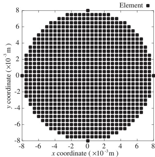
Fig. 6. Element pattern for a 797-element array.
