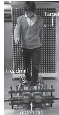
Fig. 3 Experimental site of the target on the treadmill.
