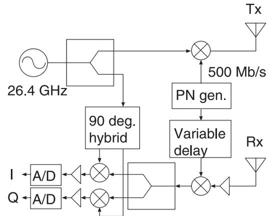
Fig. 1. Block diagram of the measurement system.
