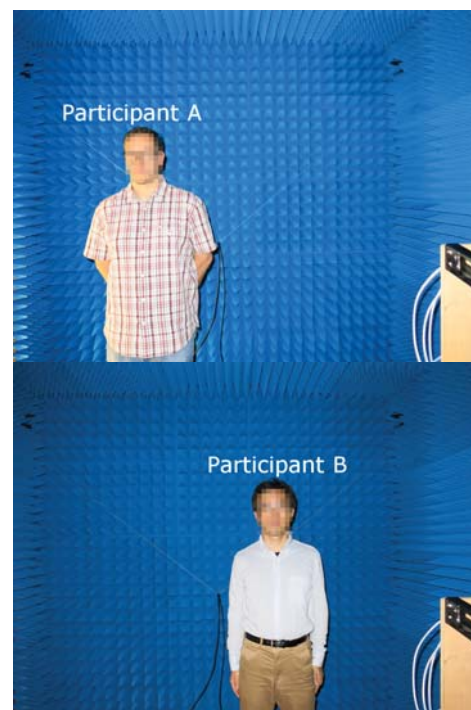
Fig. 5. Measurement scenarios with participants A and B standing in front of the antenna array.
