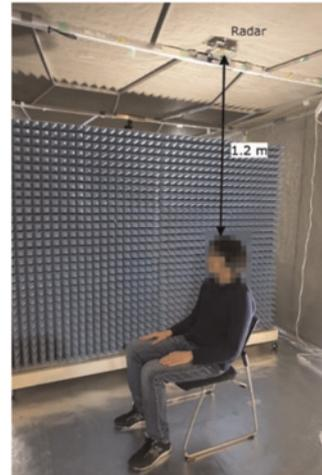
Fig. 2 Measurement setup with a radar module and a seated participant
