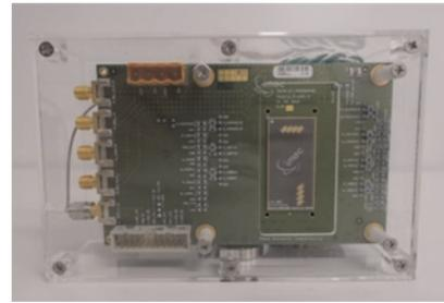
Fig. 1 79 GHz MIMO radar module developed and used in this study
