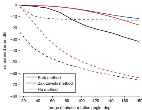
**Fig. 2** Estimated errors using three methods with a SNR of 10 dB (solid line) and 40 dB (dotted line)
