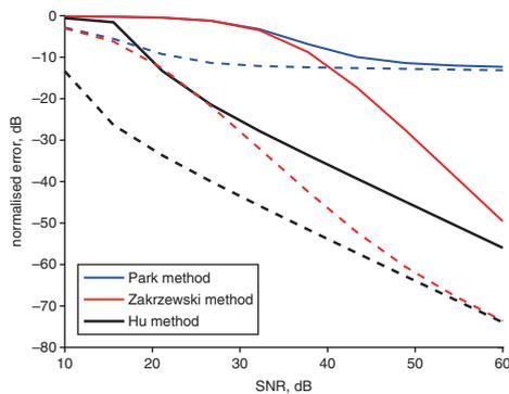
**Fig. 1** Estimated error using three methods. Phase rotation angle was  $30^\circ$  (solid line) and  $90^\circ$  (dotted line)
