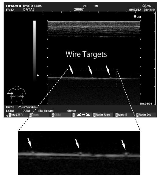
Fig 1. B-mode image of a calcification phantom.
