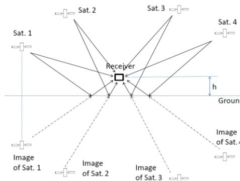
Figure 1. Schematic system model for simulation
