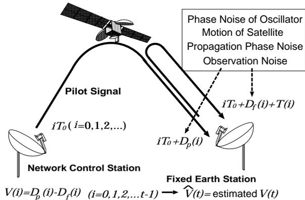
Figure 1: System model of a synchronous CDMA communication system with a GEO satellite.
