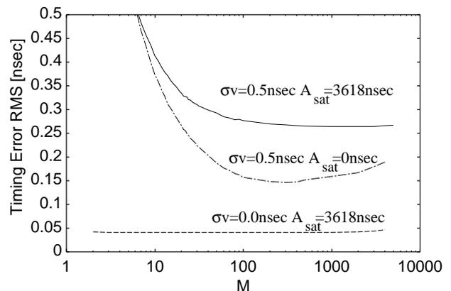
Figure 8: Relationship between RMS estimation errors and  $M$ .
