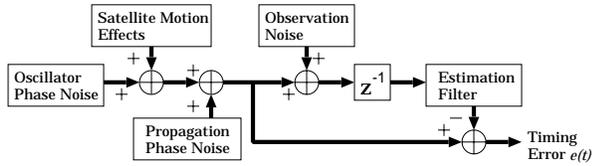
Figure 3: Procedure of computer simulation.
