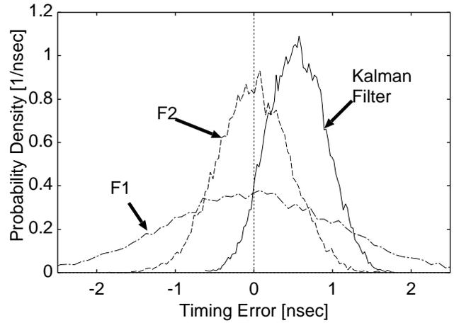
Figure 6: PDF of timing errors in three estimation methods using different filters.
