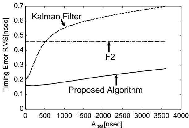
Figure 10: Relationship between RMS timing error and  $A_{\text{sat}}$  for each synchronization method.
