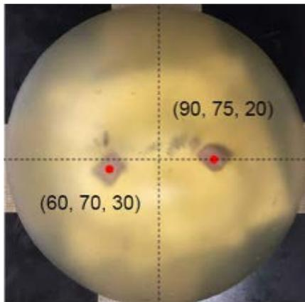
Fig. 1. Breast and cancer tissue phantom used for measurement.
