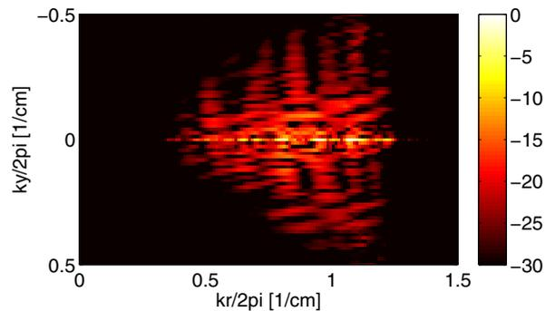
Fig. 6. Frequency-wavenumber spectrum of the frequency-domain Kirchhoff migration (in decibels). High frequency-wavenumber components are enhanced.
