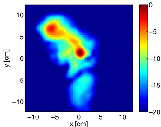
Fig. 10. Radar image generated using the proposed method (frequency-domain Kirchhoff migration) [6]. The computational time was 4.5 s.
