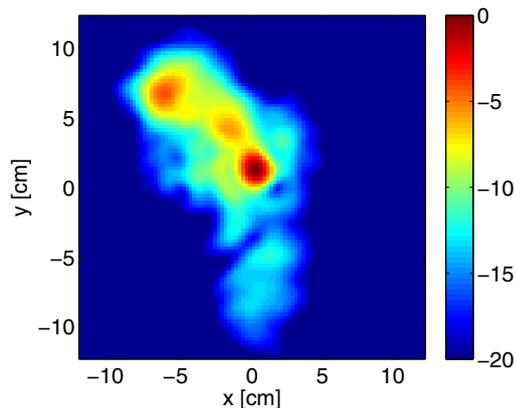
Fig. 8. Radar image generated using modified Kirchhoff migration [4]. The computational time was 1149 s.
