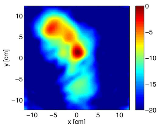
Fig. 9. Radar image generated using conventional F-K migration. The computational time was 2.5 s.
