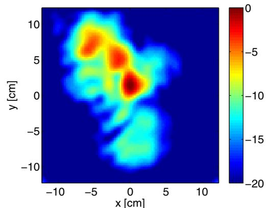
Fig. 7. Radar image generated using conventional DAS migration. The computational time was 1119 s.
