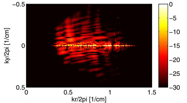
Fig. 3. Frequency-wavenumber spectrum of the conventional F-K migration (in decibels).
