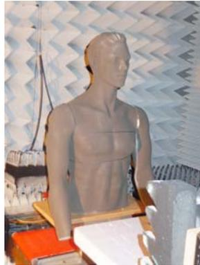
Figure 2: Metal-coated mannequin on a moving platform used in our radar measurement.
