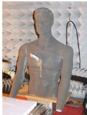
Fig. 8. A mannequin with a handgun on its chest used for our measurement.
