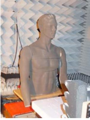
Fig. 2. Photo of metal-coated mannequin on a moving platform used for our measurement.
