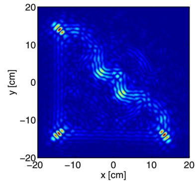
Fig. 4. Estimated target shape using the conventional migration method for target A.
