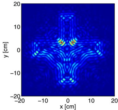
Fig. 5. Estimated target shape using the conventional migration method for target B.
