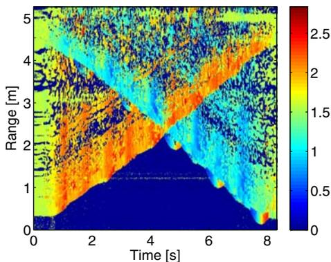
Fig. 7. Texture flow angle of the time-range signals (in rad).
