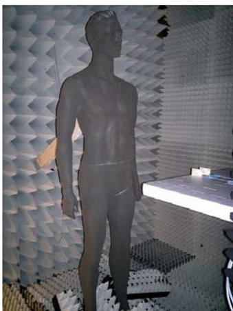
Fig. 6. Metal-coated mannequin for the measurement.
