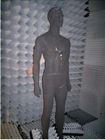
Fig. 3. Experimental setup with a mannequin and a weapon.
