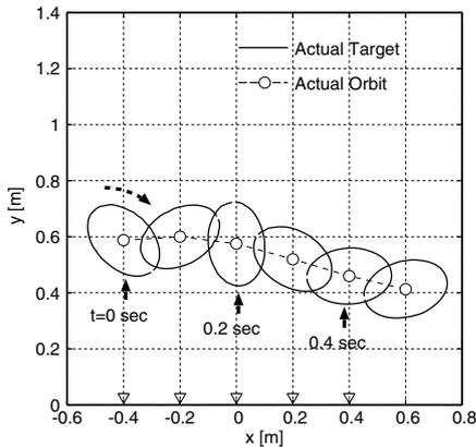
Fig. 2. Assumed elliptical target shape and motion with rotation.
