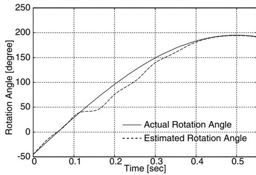
Fig. 9. Actual and estimated rotation angle using the proposed method ( $\delta = 0.1$ ).
