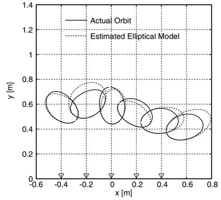
Fig. 7. Estimated elliptical models for non-elliptical target ( $\delta = 0.1$ ).
