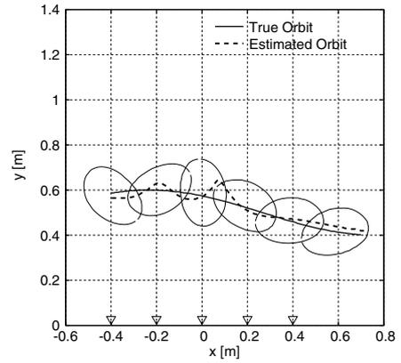
Fig. 8. Actual and estimated translation orbits using the proposed method for a non-elliptical target ( $\delta = 0.1$ ).
