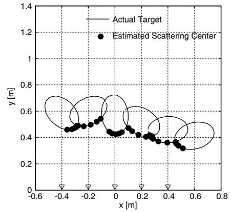
Fig. 3. Estimated scattered points for an elliptical target.
