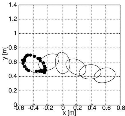
Fig. 10. Actual and estimated target shapes for a non-elliptical target using the proposed method ( $\delta = 0.1$ ).
