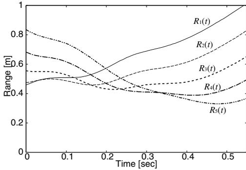
Fig. 6. Measured range data using 5 antennas for a non-elliptical target  $\delta = 0.1$ .
