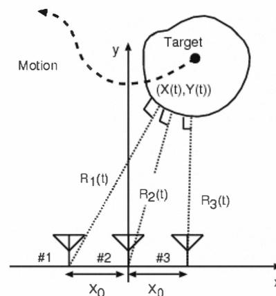
Fig. 1. 2-dimensional system model.
