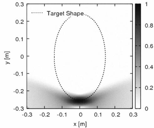
**Fig. 8.** Target shape estimated using a conventional method.
