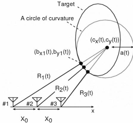
Fig. 2. Parameters of a circle of curvature.
