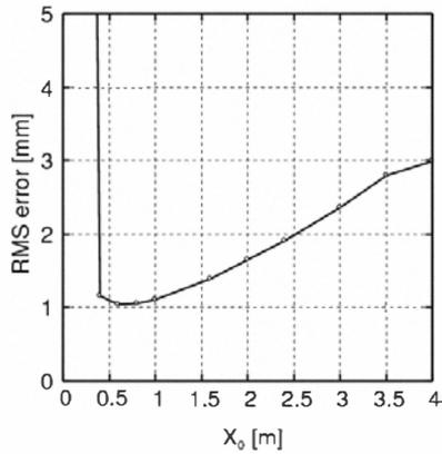
**Fig. 7.** RMS error versus the antenna distance  $X_0$
