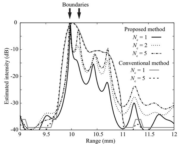
Fig. 6. Estimated intensities in a scan line calculated by the proposed method and a conventional method. An agar membrane about 0.2 mm thick was located at 1 cm depth.  $N_c$  denotes the number of coherent integration for the improvement of signal to noise ratio of IQ data. Arrows indicate the boundary ranges.
