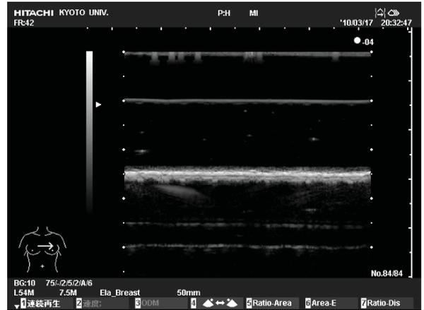
Fig. 4. B-mode image of a gelatin block with an agar membrane about 0.27 mm thick at 1 cm depth.
