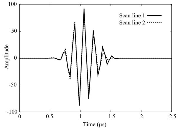
Fig. 2. Pseudo-double RF data converted from the two IQ data of the echoes from the boundary.
