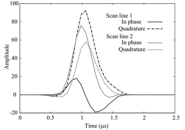
Fig. 1. IQ data of the echoes from a boundary between gelatin and agar in two scan lines.
