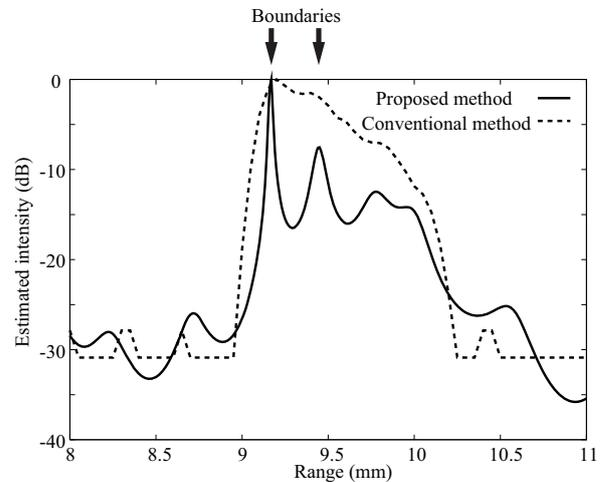
Fig. 5. Estimated intensities in a scan line calculated by the proposed method and a conventional method. An agar membrane about 0.27 mm thick was located at 1 cm depth. Arrows indicate the boundary ranges.
