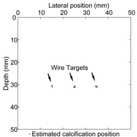
**Figure 6.** Estimated wire target positions selected using the proposed method.
