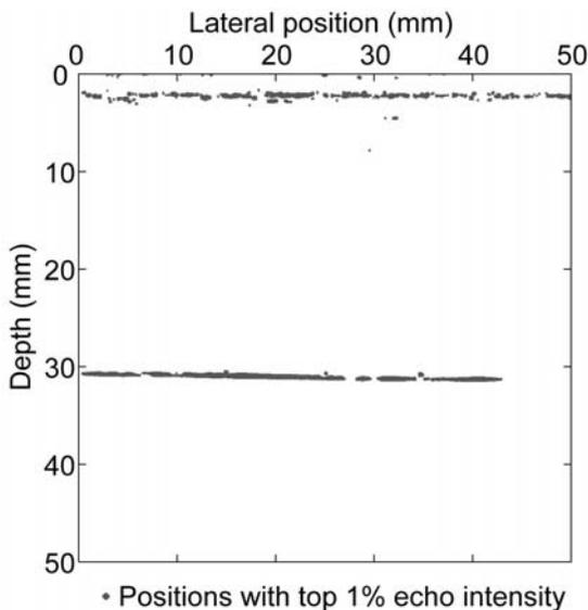
**Figure 4.** Candidates for wire target positions with the top 1% signal intensity.
