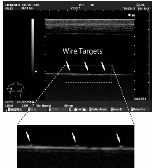
**Figure 3.** B-mode image of the calcification phantom with a swine fat layer. The diameters of wires are 0.2, 0.29 and 0.4 mm in left to right order.
