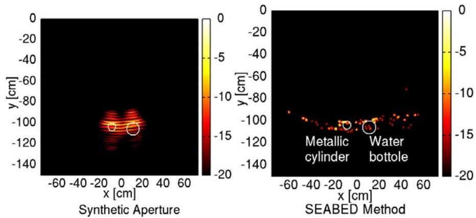
Fig. 5. Images by synthetic aperture and SEABED for multi-static radar data with 2 targets located very close together.
