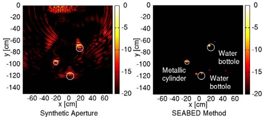
Fig. 1. Images by synthetic aperture and SEABED for mono-static radar data with 3 targets.
