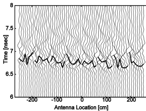
Figure 6 Received signals and the mistakenly extracted inaccurate quasi-wavefront.
