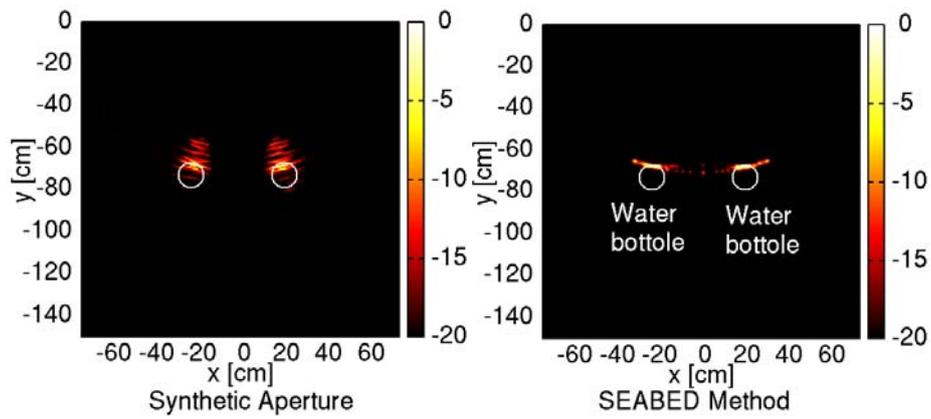
Fig. 4. Images by synthetic aperture and SEABED for multi-static radar data with 2 targets located close together.
