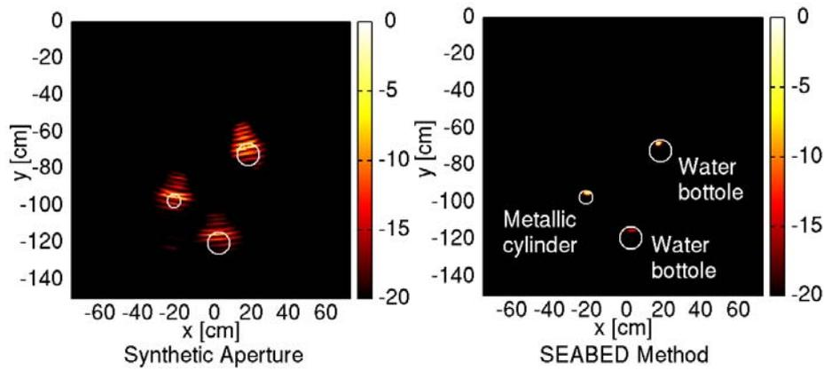
Fig. 2. Images by synthetic aperture and SEABED for multi-static radar data with 3 targets.
