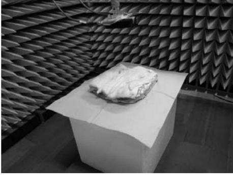
Figure 5: Experimental site for UWB radar with an anterior abdominal wall.
