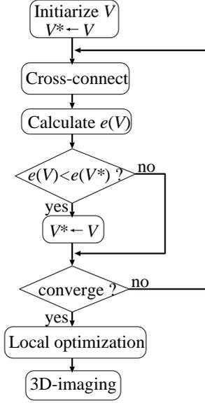
Fig. 8. Proposed extraction method for quasi-wavefronts.
