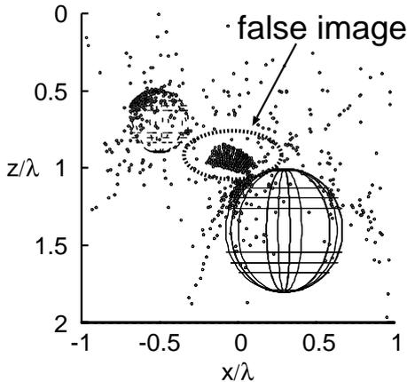
Fig. 5. Estimated target shape using the sequential subtraction method (without noise).
