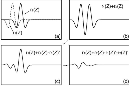
Fig. 3. Interference reduction process using the sequential subtraction method.
