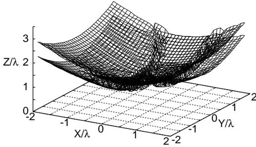
Fig. 4. Estimated quasi-wavefronts using the sequential subtraction method.
