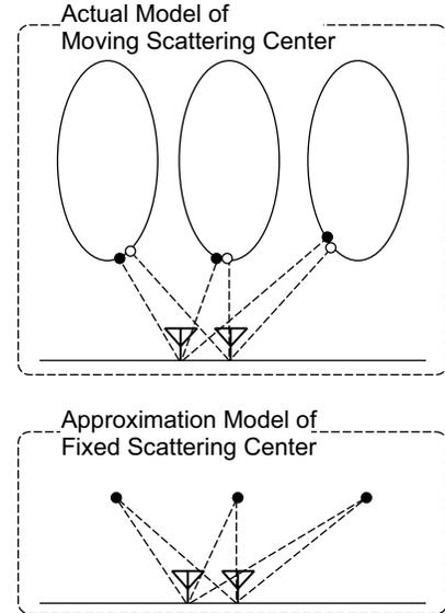
Fig. 3. Actual and approximation models of scattering center.
