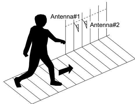
Fig. 1. Antenna arrangement for imaging human bodies.
