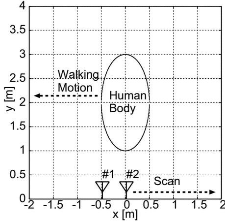
Fig. 2. 2-dimensional system model.
