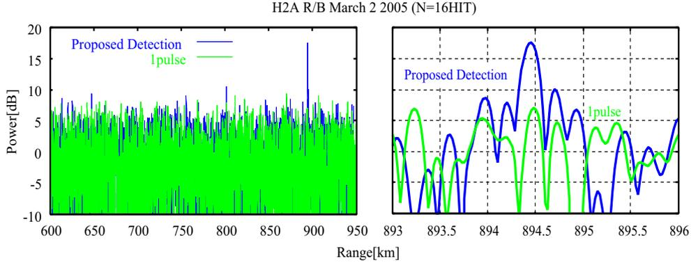
Figure 7. Example of Proposed Detection Method Applied to the Real Data.
