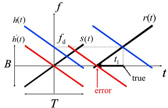
Figure 1. Liner-chirp Pulse Compression.
