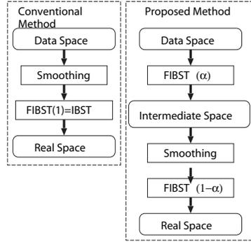
Figure 4: The procedure of the proposed algorithm.
