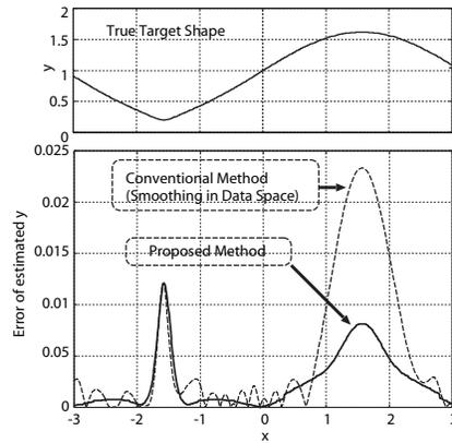
Figure 6: Estimation accuracy by SEABED algorithm with each stabilization method.
