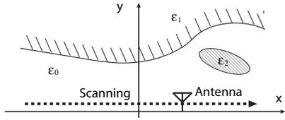
Figure 1: System model and antenna scanning.
