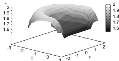
Fig. 1. Estimated target shape by SEABED algorithm with FDTD data. Computation time for the entire imaging is 13msec.
