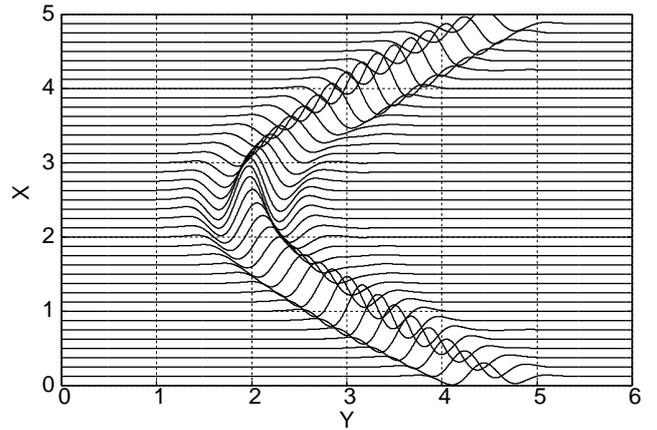
Fig. 2. Output of the matched filter for the transmitted waveform.
