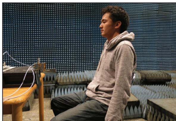
other hand, whilst the echo phase is sensitive to small displacements in the patient, the echo power is near constant. This causes the signals containing information about vital signs to move along a circle in the I-Q plane (a complex plane displaying the phase and amplitude of the received electromagnetic waves). The static clutter signals in contrast, appear at the centre of such circles. In their Letter, the authors looked at three existing techniques to
