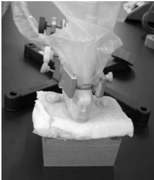
Fig. 2 Calcification phantom with a swine skin and subcutaneous fat layer
