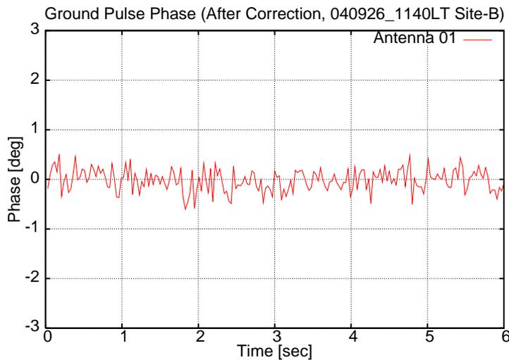
Figure 5.9: Phase of ground pulses after the compensation process. Fluctuations are removed compared to Fig. 5.7(right).
